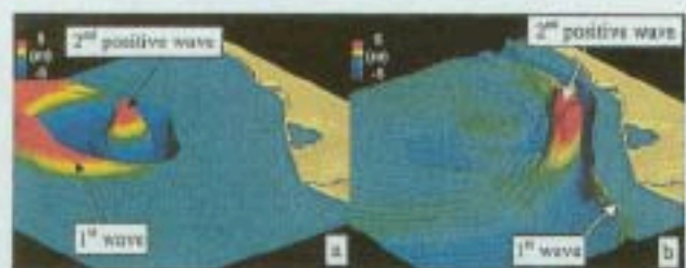
Figure 4. Snapshots of the computed water surface at t=90 s (a) and t=360 s (b) after the slide initiation. Same horizontal dimensions as in Fig. 3. Vertical scale is exaggerated by a factor 750 with respect to horizontal scale.
