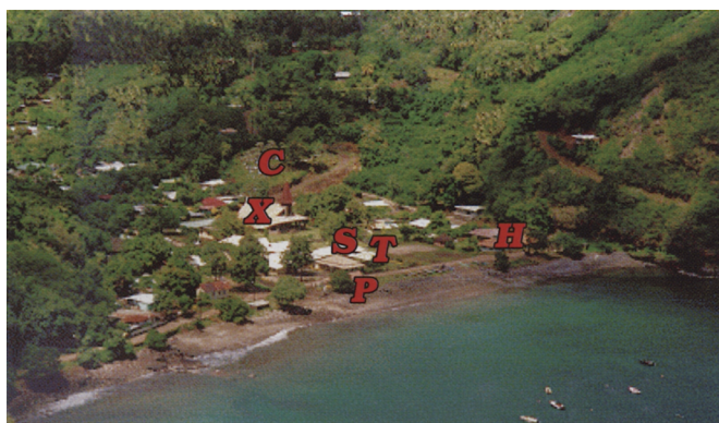
▲ Figure 8. View of the village of Vaitahu on Tahuata Island (Marquesas), illustrating hazardous waterfront development. The 1946 wave penetrated inland to a location along the back wall of the present church (X; built in the 1980's), 145 m from the shoreline. Note the hazardous location of the post office (P), town hall (T), elementary school (S), and hospital (H). Ironically, only the cemetery (C) is safely located on a hill.
